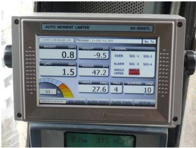
Fig. 1. Monitor for an anti-collision system.
