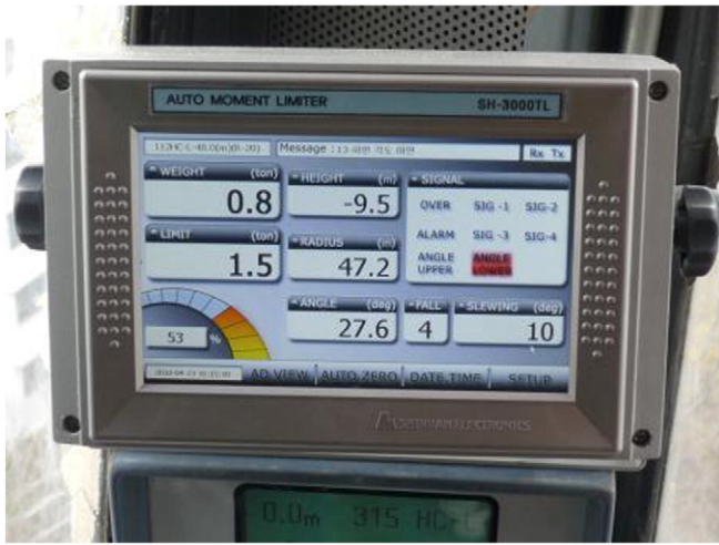
Fig. 1. Monitor for an anti-collision system.
