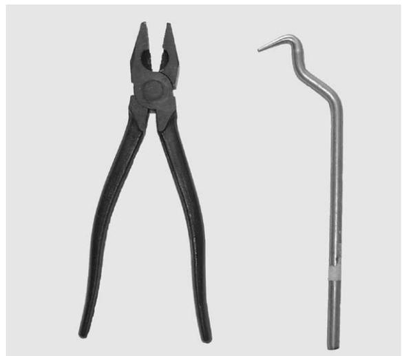
Fig. 1. Pliers and wire-tying hook.
