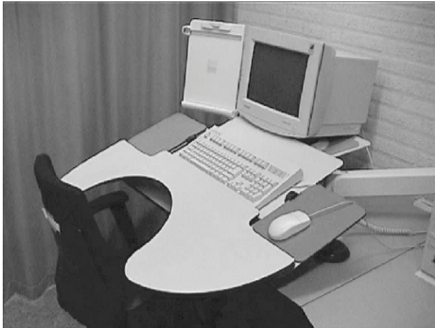
Fig. 1. The Up-Line: characteristics of the Up-Line are the inclined work area and the position of the keyboard close to the screen.
