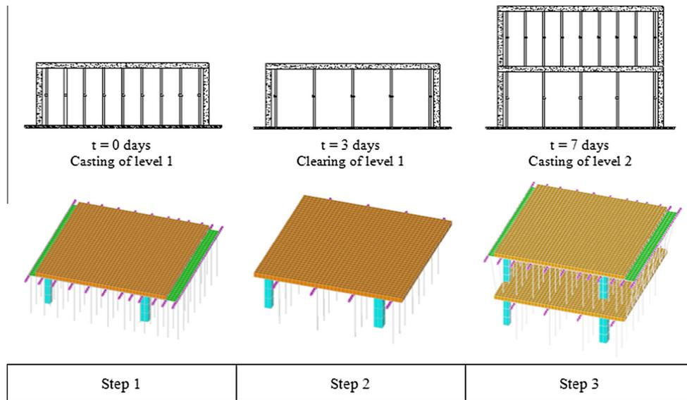
Fig. 2. Construction phases and load steps in experimental building (1).
