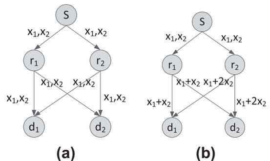
**Fig. 1.** A flood-based application in which node  $s$  floods packets  $x_1$  and  $x_2$  in the entire network: (a) transmissions when network coding is not used (a total of 6 packet transmissions); (b) transmissions when network coding is used (4 packet transmissions).
