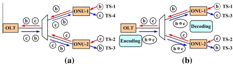
Fig. 1. Operation principle of inter-ONU communication in all-optical VPN. (a) Traditional TDM-VPN and (b) all-optical VPN with network coding.
