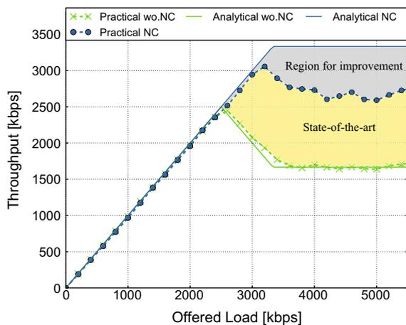
Fig. 1. Discrepancy between analytical results, based on [8], and practical results from [14]. Here, we clearly see the difference when using inter-session NC while there is a perfect match for the pure forwarding.
