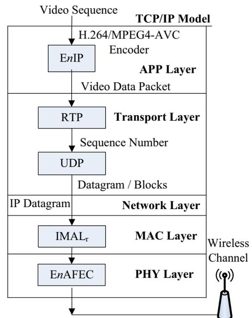
Fig. 1. TCP/IP model for multi-layer structure.
