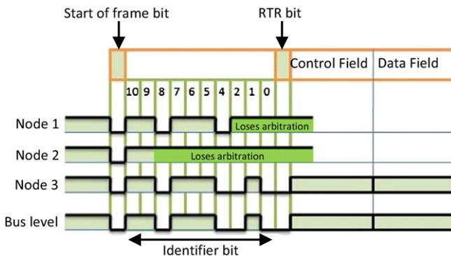
Fig. 1. CAN bus arbitration example.
