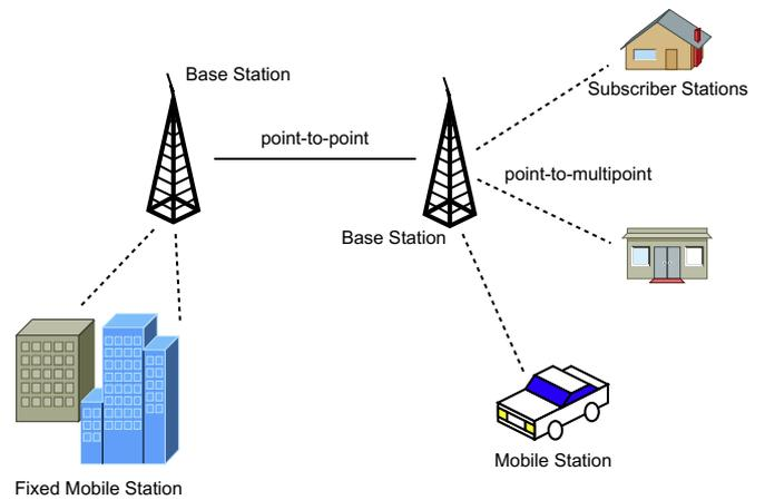
**Fig. 1.** Deployment of WiMAX networks.
