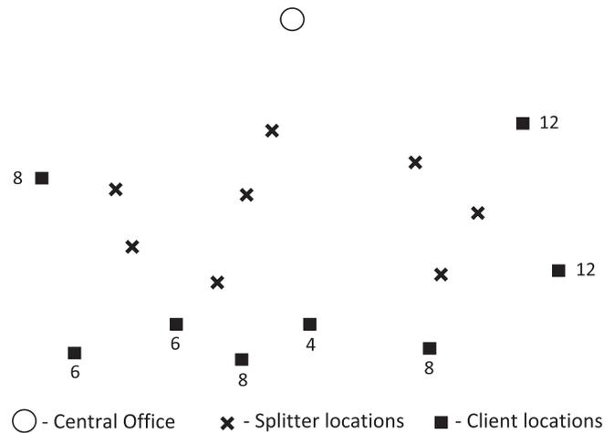
Fig. 1. Central office, splitter and client locations.
