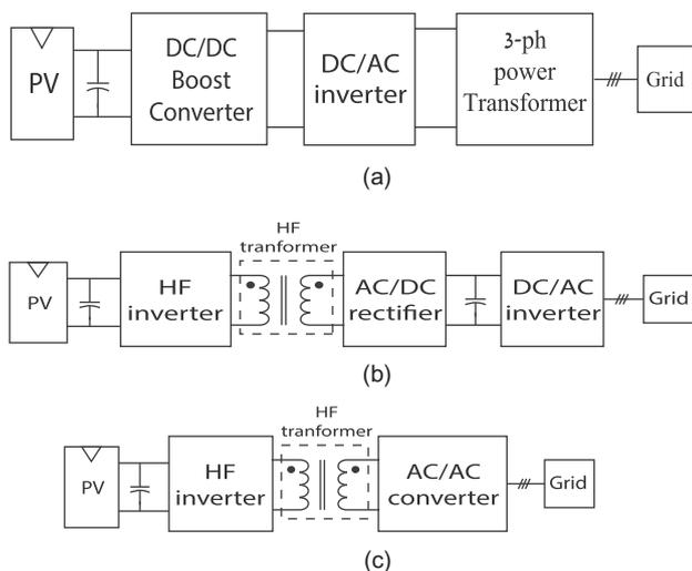
Fig. 1. PV-grid interface systems: (a) traditional, (b) HFDC link, (c) HFAC link.
