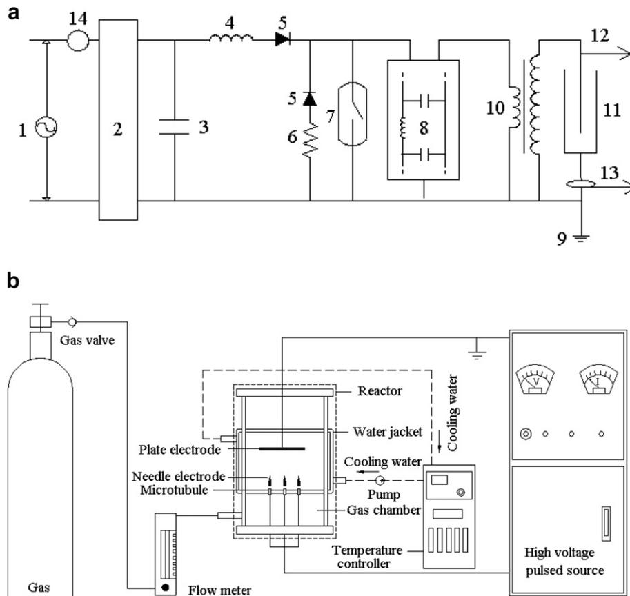
Fig. 1. (a) The topology circuit of pulsed high voltage source. (1) AC input (0–380 V); (2) DC high voltage source; (3) capacitor; (4) inductance; (5) diode; (6) resistance; (7) thyatron; (8) Blumlein pulse forming network; (9) earth point; (10) pulse transformer; (11) pulsed electrical discharge reactor; (12) voltage sampling; (13) current sampling; and (14) AC wattmeter. (b) The diagrammatic sketch of experimental apparatus.
