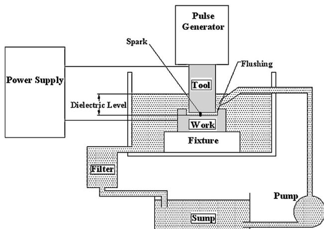
Fig. 1 – Schematic diagram of EDM process.
