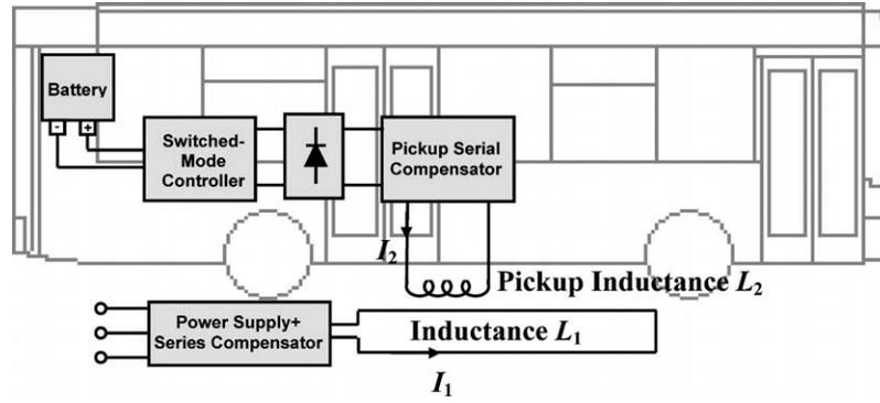
Fig. 1. Scheme of the ICPT battery charger.
