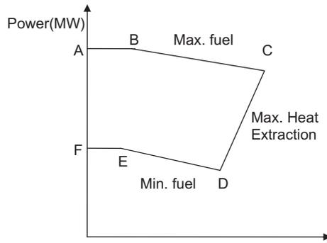
Fig. 1. Heat-power feasible operation region for a cogeneration unit.
