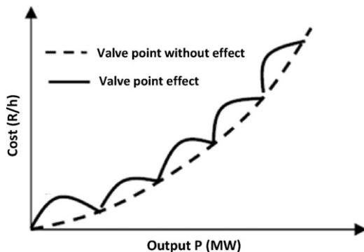
Fig. 1. Input–output characteristics of the generation units.
