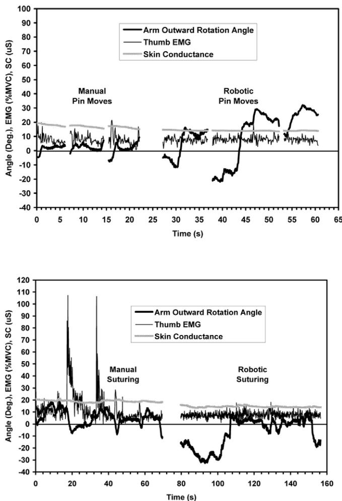
**FIG. 1.** Top: A subject's time plots of right arm outward rotation angle (abduction), thumb electromyography, and skin conductance for the three Pin Move trials laparoscopically (left) and robotically (right). Bottom: A subject's time plots of right arm outward rotation angle (abduction), thumb electromyography, and skin conductance for the Suture task laparoscopically (left) and robotically (right). The individual recordings were concatenated for these figures.
