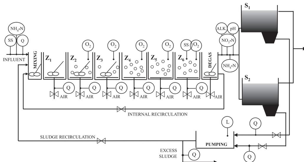
Fig. 1. Simplified layout for a single ASP line and location of on-line measurements.
