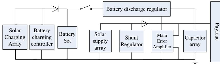
Fig. 1. Diagram of the satellite power subsystem and its sensor deployment.
