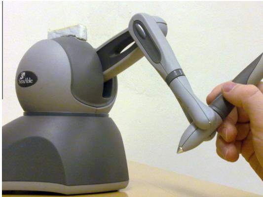
Fig. 1. Example of haptic device – Phantom Omni®.
