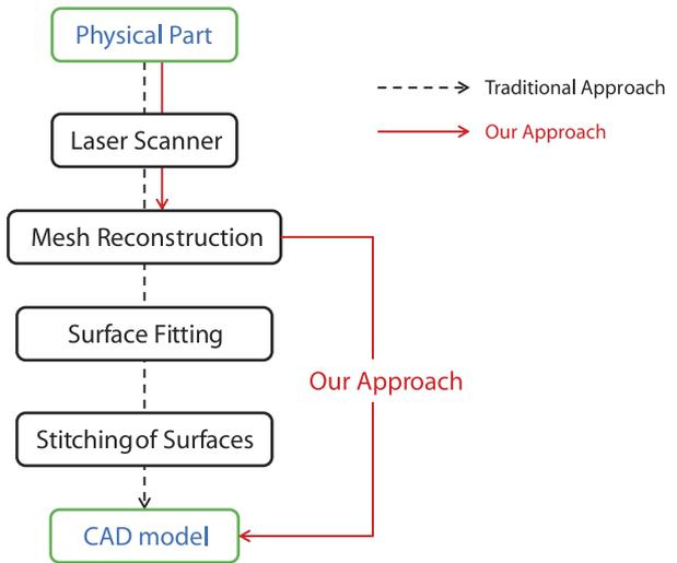
Fig. 3. Traditional reverse engineering pipeline versus our approach. We obtain the direct parameterization of CAD model by completely skipping the reconstruction of surfaces.
