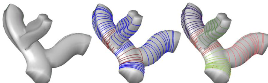
Fig. 2. Volumetric understanding: (From Left to Right) mesh model, PCS generation (full cross-sections are shaded in blue and partial cross-sections in brown), and sets of PCS representing different sweep segments obtained after clustering. (For interpretation of the references to colour in this figure legend, the reader is referred to the web version of this article.)
