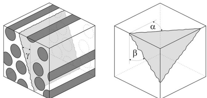
Fig. 1. Description of fracture plane orientations in transversely isotropic materials (left) and isotropic materials (right).
