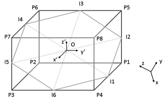
Fig. 2. Exemplary fracture plane in a finite element for the case of 6 intersections.
