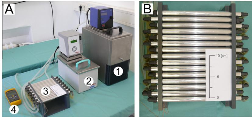
**Fig. 1.** Experimental setup for eliciting the thermal grill illusion. (A) Water is cooled and heated, respectively, in two thermostats (1, 2) and pumped through every other bar in the grill device (3 and B). At the measuring site where the palm is being placed (3), the temperature is being measured by a digital thermometer (4).
