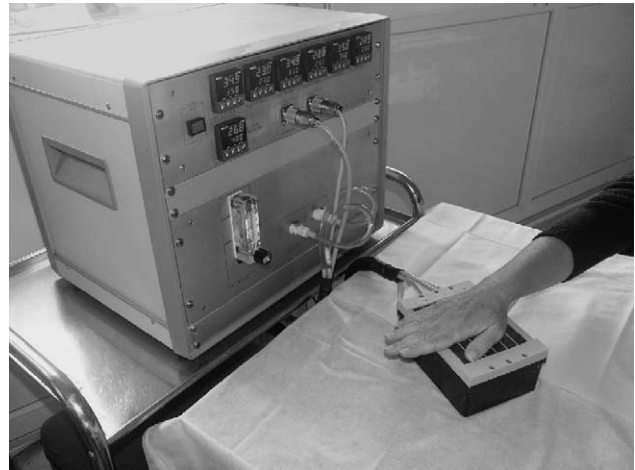
Photograph. The volunteers applied their right hand palm on the thermode (i.e. thermal grill) orthogonally to the long axis of the bars. The thermode was composed of six bars (1.2 × 16 cm) covered with a copper plate, spaced 2 mm apart for thermal isolation. The control unit allowed to set the temperature of alternate (even- and odd-numbered) bars by means of Peltier elements (3 per bar).
