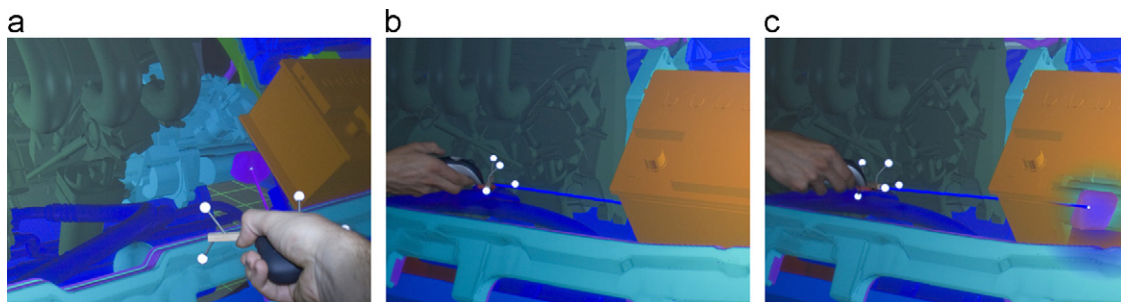
Fig. 1. The first two images (a, b) illustrate the issue of interpersonal occlusion between two tracked users in a multi-user VR system: an object that is fully visible to one user (a) cannot or only partially be seen from other viewpoints (b). Show-through techniques can improve target discovery in such situations by showing the indicated object through the occluding environment (c).
