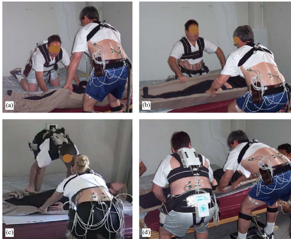
Fig. 1. Lateral transfers being performed with the bedsheet only (a), the dual rod (b), the bridgeboard (c), and the single rod (d). All the two-sided transfers were performed once with the person in the bedside role kneeling (a and b) and once with the person in the bedside role standing (c). With the single-rod transfers the “bedside” FFP was positioned alongside the stretcher-side FFP.
