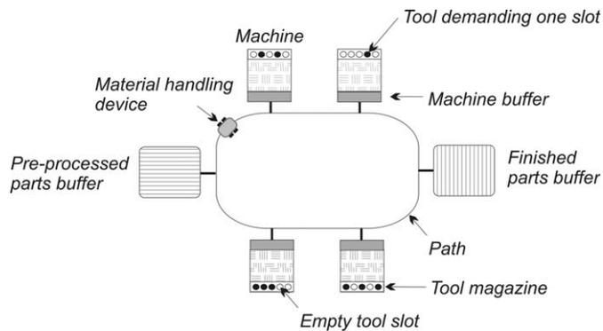
**Fig. 1.** Schematic representation of an FMS environment (four machines, tool magazines of five slots each, one material-handling device, and buffers for pre-processed and finished parts as well as machine buffers).
