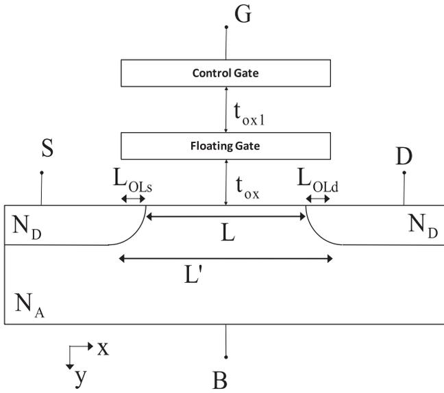
**Fig. 1.** Cross-sectional representation of an n-channel floating-gate memory cell, where  $t_{ox1}$  – control gate (CG) to floating gate (FG) oxide thickness,  $t_{ox}$  – FG to substrate oxide thickness,  $L_{OLd}$ ,  $L_{OLs}$  – drain and source overlap lengths,  $W$ ,  $L'$  – cell width and length,  $L$  – channel length.
