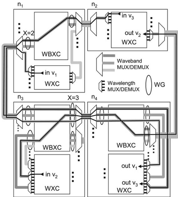
Fig. 1. Multi-granular nodes and waveband tunnels.
