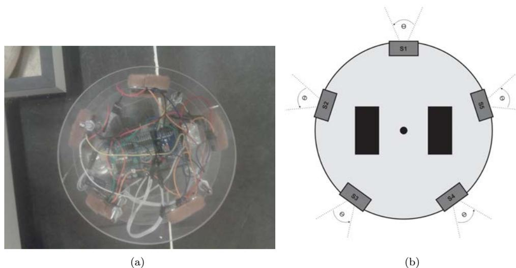
Figure 1: Real (a) and simulated (b) robot configuration.
