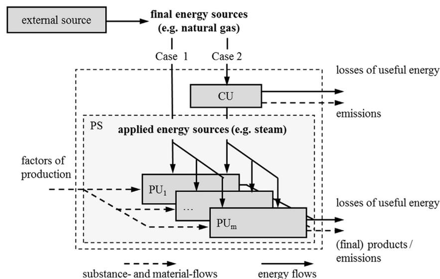
Fig. 1. Energy supply for production systems (following [4]).
