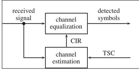
Fig. 1. Channel estimation and equalization in TDMA systems.
