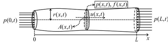
**Fig. 1.** An axisymmetric vessel with radius  $r(x, t)$  and fixed length  $L$ . The direction of the average blood velocity  $u(x, t)$  is along the axis of the vessel. The viscous effect  $f(x, t)$  arises from the shear stress on the vessel wall.
