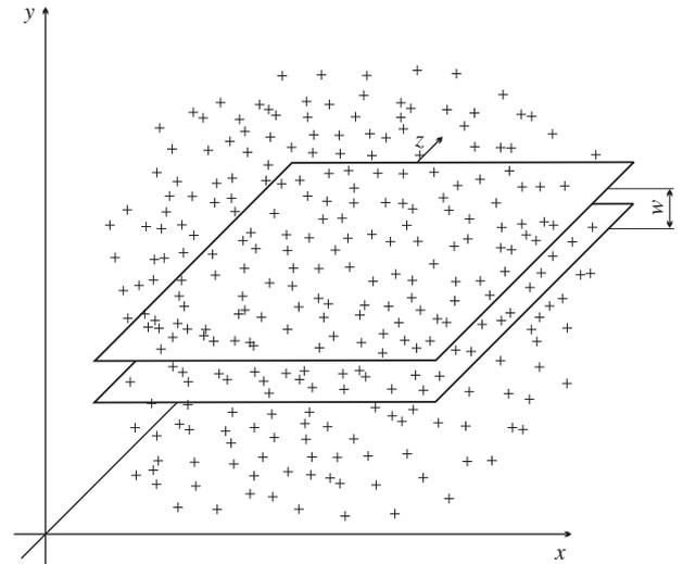
Fig. 1. Bounding box of input points is divided into slices of the width  $w$ .
