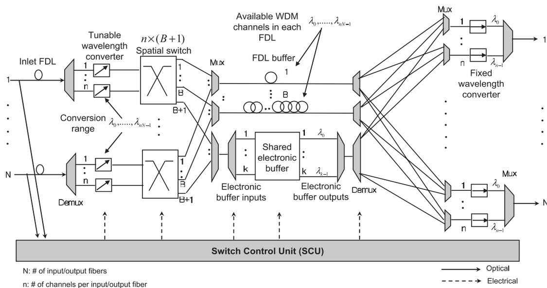
Fig. 1. OPS architecture with a hybrid buffer.
