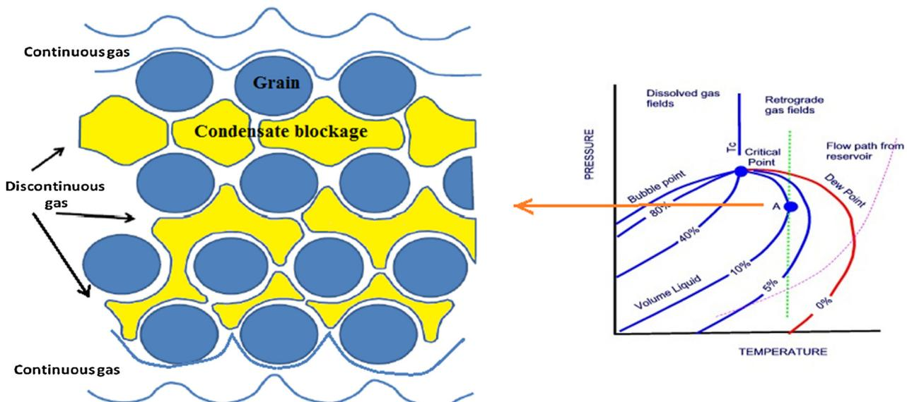
Fig. 1. Condensate block formation in pore spaces of reservoir.
