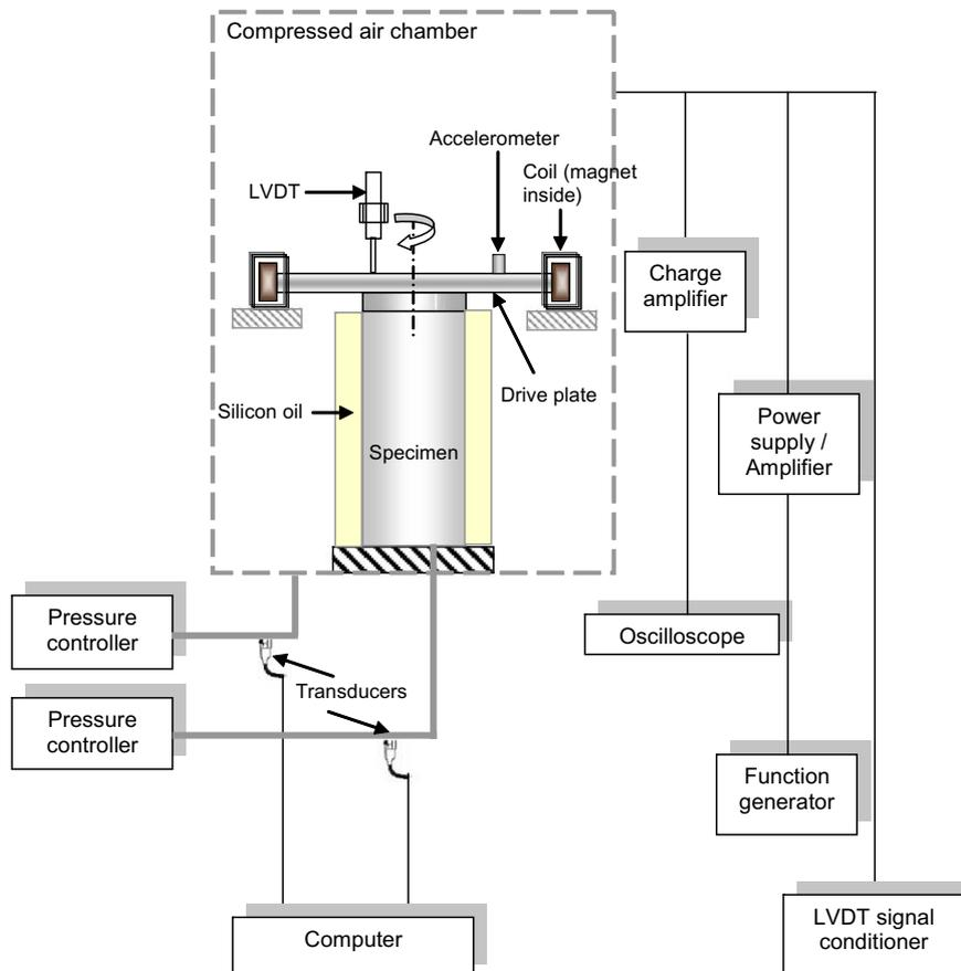
Fig. 1. Simplified diagram of the resonant column testing apparatus used in the experimental study.
