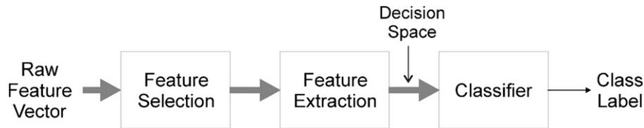
Fig. 1. Prototypical pattern recognition system.
