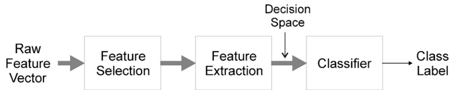
Fig. 1. Prototypical pattern recognition system.
