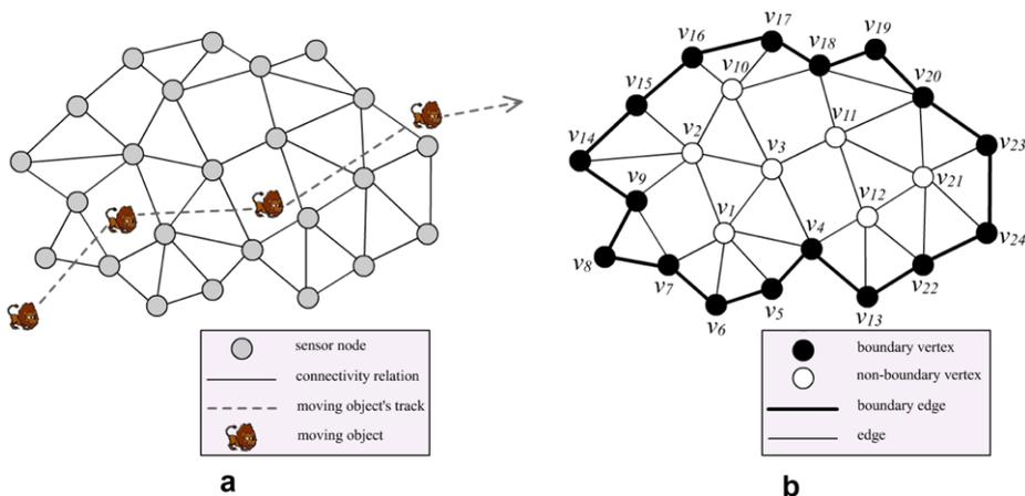
Fig. 1. (a) An overview of a WSN and (b) the corresponding graph model for the WSN.
