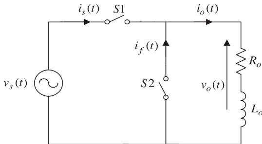
Fig. 1. PWM AC/AC voltage converter with bi-directional switches.
