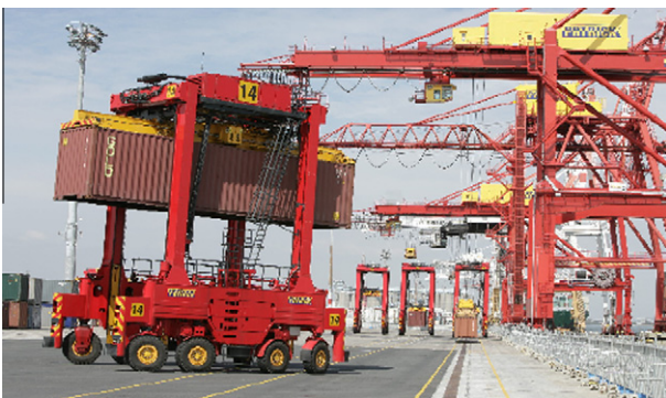
Fig. 2. Fully autonomous straddle carrier transporting a 40-foot container from the quay-side as part of a buffer-to-yard task.
