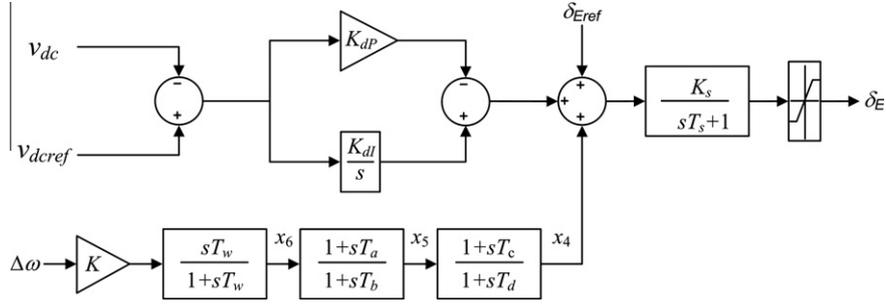
Fig. 1. Lead-lag controller with DC voltage regulator.
