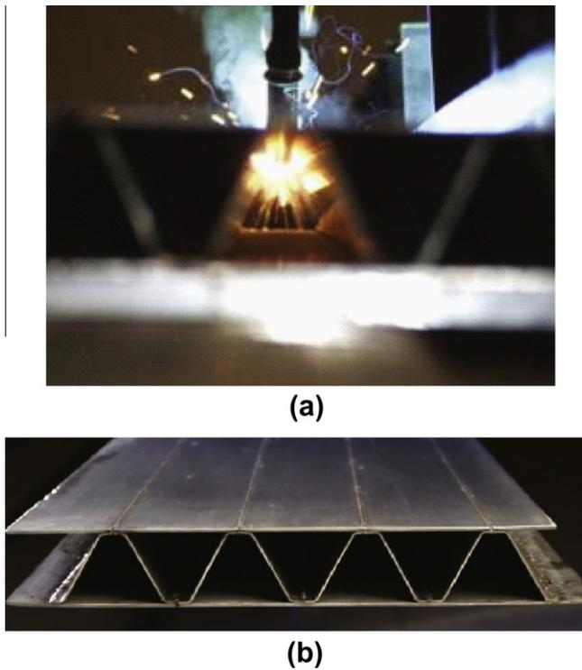
**Fig. 1.** Fabrication of laser welded steel sandwich panels, (a) laser stake welding of prismatic cores to facings and, (b) post production laser welded sandwich panel (Applied Thermal Sciences Inc., Sanford, Maine, USA).
