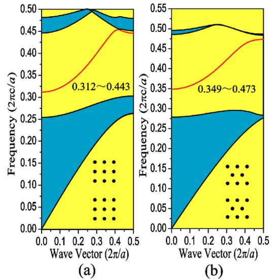
**Fig. 2.** TM band structure for different PC waveguides as shown in the inset (a) square-lattice GaAs PC waveguide and (b) triangular-lattice GaAs PC waveguide.
