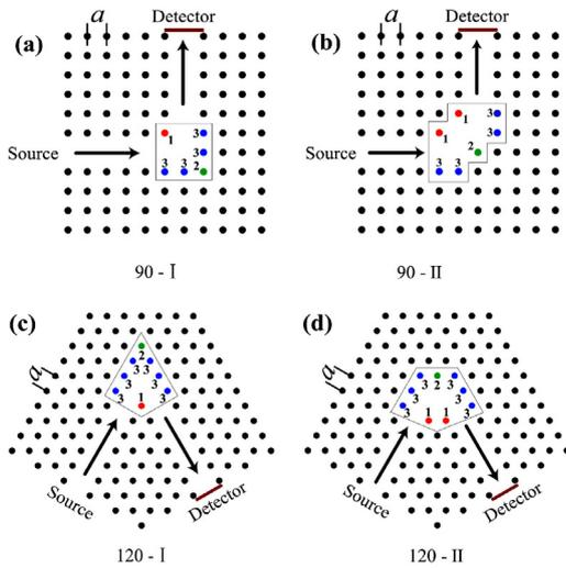
**Fig. 1.** Scheme of PC waveguide bend models studied in this paper: (a) and (b) represent  $90^\circ$  bends with different corner geometries, (c) and (d) represent  $120^\circ$  bends with different corner geometries.
