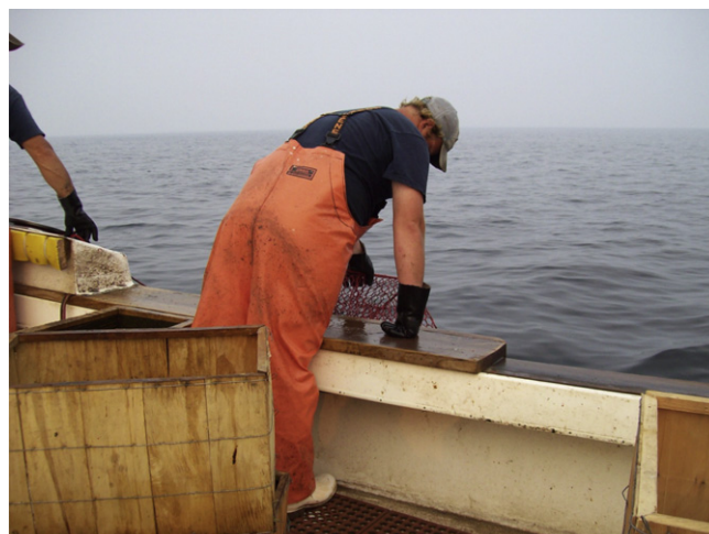
Fig. 2. The Crab Pot Ramp intervention mounted to the side of the fishing boat.
