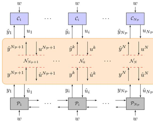
**Fig. 1.** The networked control setup considered in this paper, in which  $N_p \in \mathbb{N}$  (coupled) plants  $\mathcal{P}_i$  and their controllers  $\mathcal{C}_i$ ,  $i \in \{1, 2, \dots, N_p\}$ , are connected via  $N_N \in \mathbb{N}$  communication networks  $\mathcal{N}_k$ ,  $k \in \{N_p + 1, N_p + 2, \dots, N_p + N_N\}$ . The variable  $w$  denotes the disturbance acting on the plants.
