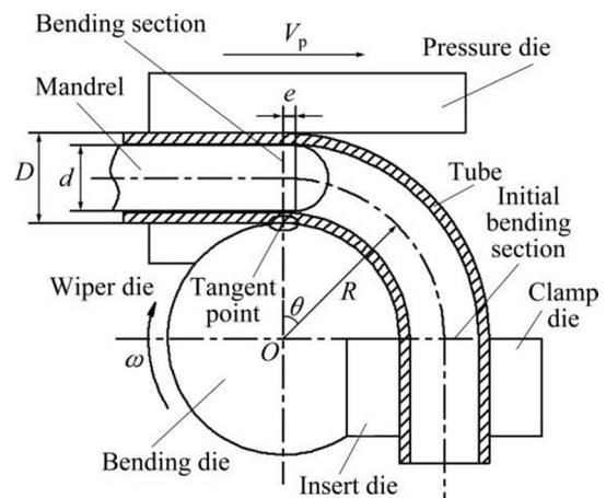
Fig. 1 Schematic diagram of tube NC bending
