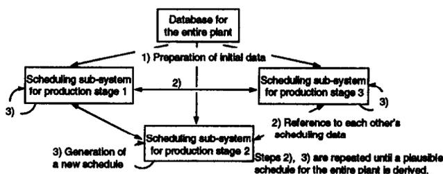
Fig. 1. Autonomous decentralized scheduling system.
