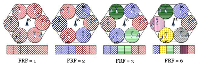
Fig. 2. Frequency reuse patterns.
